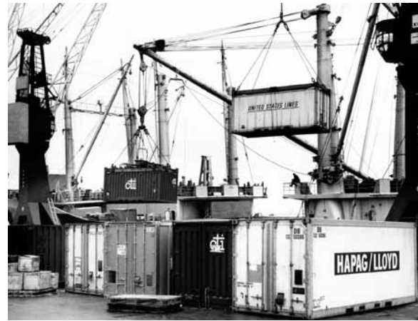
Unloading containers with shipboard gear in Neustädter Hafen, Bremen, 1967
