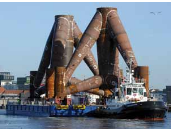
Tripods on OFFSHORE BHV I pontoon on the way to ABC peninsula in Bremerhaven
